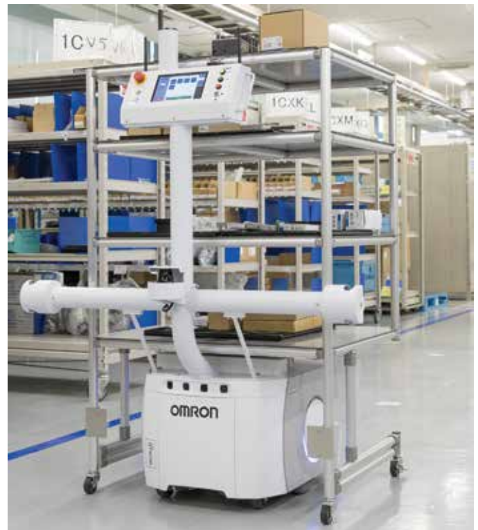
Mobile robots boost flexibility by transporting materials throughout the factory using an intelligent self-guiding mechanism.
